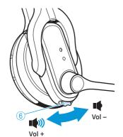
The volumes can be adjusted in several steps. When the minimum or maximum volume is reached, you hear a double beep in the headset.
