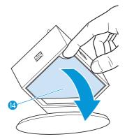
▶ Remove the cover [4] by inserting a finger into the recess as shown.
