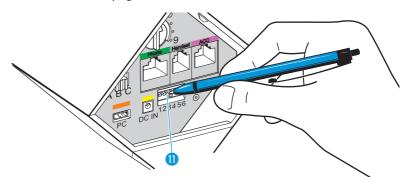
Use a pointed object (e.g. a pen) to set the DIP switches to the desired position.
