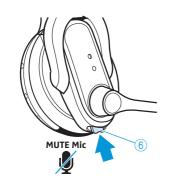
To mute the headset's microphone during a call (the LINK LED 4) on the base station lights up blue):
