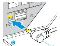
Connect the DC IN connector 6 of the power supply unit to the DC IN socket 12.
