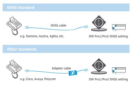
If your telephone has a built-in electronic hook switch supporting the DHSG or the any other hook switch standard (except for the MSH standard):
